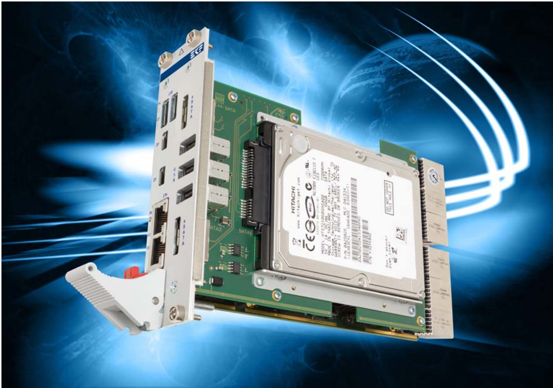
SC3-LARGO w. C44-SATA Mezzanine Module 8HP Assembly
