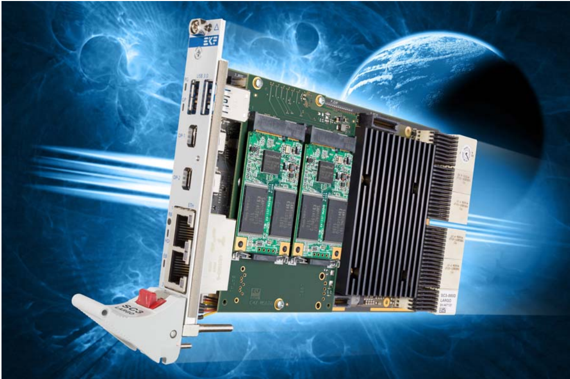
SC3-LARGO w. C47-MSATA Mezzanine Module 4HP Assembly
